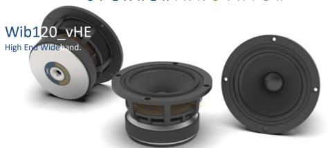
Wib120\_vHE is a modern wide band, allying low frequency extension and linear frequency response up to 22kHz. The cone (exponential profile) is made of mixed cellulose and glass fiber, with specific damping applied on the back of the membrane to minimize sound coloration.
