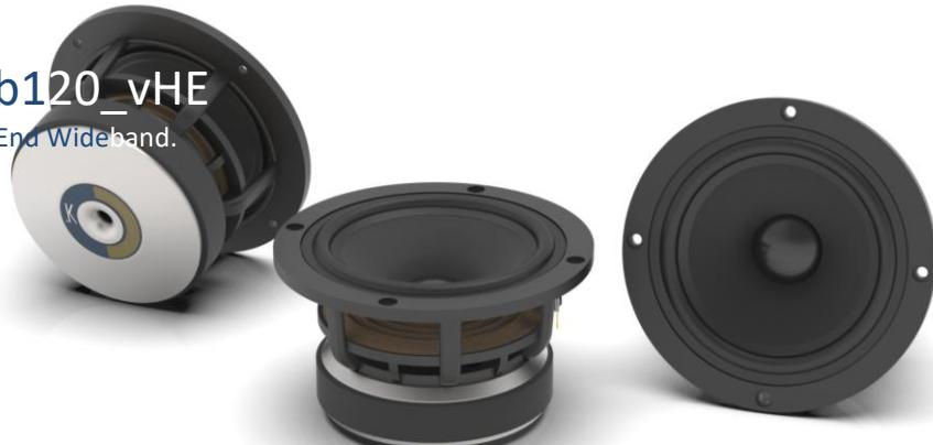
Wib120\_vHE is a modern wide band, allying low frequency extension and linear frequency response up to 22kHz. The cone (exponential profile) is made of mixed cellulose and glass fiber, with specific damping applied on the back of the membrane to minimize sound coloration.
