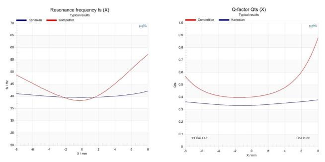
Due to suspension stiffness variation (increasing), the resonance frequency increase as well. In red, the competitor has Fs very close to the expected 40Hz value, and it remains true over +/-4mm, considering 10% tolerance during the production assembling. Nevertheless, the Fs reaches 56Hz at+8mm excursion, which doesn't provide the same performances in low frequency anymore.
