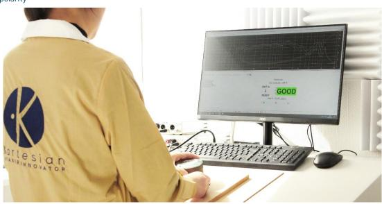
For every single loudspeaker produced, which succeed the final QC, there is a unique identification number, stored in our database. This identification number, printed and sticked on each product, is linked with parts batch in our stock for full assembling traceability.
